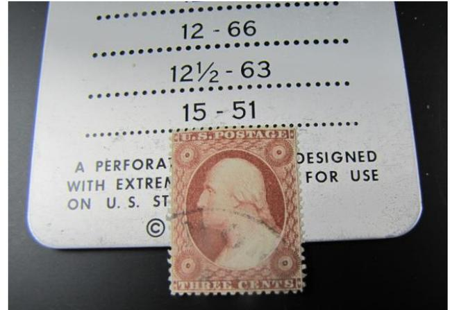
If, on the other hand, the "51" is correct (i.e., a hole separation of 0.051"), then the calculated perf is 15.44, and the Kiusalas reading should be listed as 15½-51, not 15-51. This collector believes that 15½ is the correct gauge for this issue, and therefore that the correct Kiusalas reading should be listed as 15½-51.
